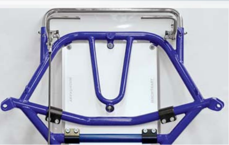
The FIA1SE kart with revised chassies geometry and the second front torsion bar.
