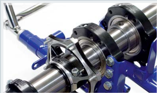
The new rear axle with modified bearing seat fixation improves driving out of the corners at a higher speed level.
